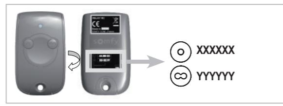
**⚠ Each remote control button code must only be used for saving a single motorisation. If the code is used to save several motorisations, the home automation box will control all these motorisations at the same time.**
