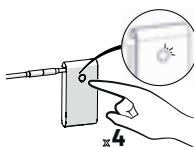
Press the module key four times, the light will flash quickly. It indicates motor enters matching status. The light will disappear once module matching done.
