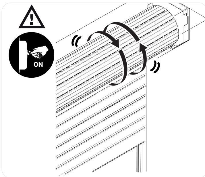
*Check that the connection has been made correctly. Incorrect connection may render the motor inoperative and the previous step will not be performed.*
