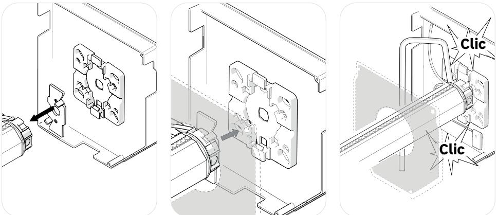
First, snap the mounting bracket into the motor head in the position shown above and then insert the end of the product containing the power and communication cables into the mounting base supplied, then insert the retaining clip until you hear it click into place.
