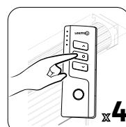
1) Press the stop button on the remote control four times.
