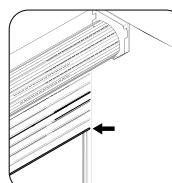
1) Position the shutter according to the desired third limit.
