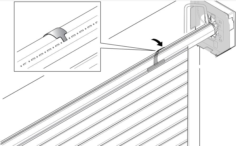
Fix the shutter slats to the shaft, maintaining the same distance as before dismantling.
