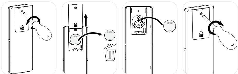
Using a Phillips screwdriver, remove the battery cover, replace the old battery with one of the same type, slide the cover on and then screw it shut.
