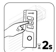
5) Long press emitter's stop button for 2S, the motor will run to the third limit position
