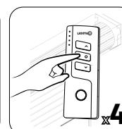
2) Once you have set the top and bottom limits. Press the stop button on the remote control four times.
