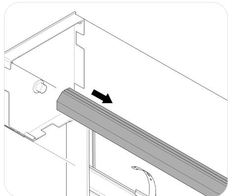
When replacing the motor, take care to protect the electric cable to avoid damaging it when removing and inserting the motor into the shutter shaft.
